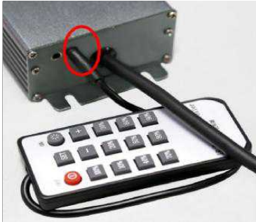
Insert the signal terminal into the bigger hole at the driver output side
